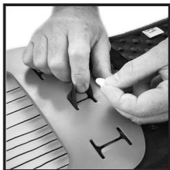
2. place standard rivet head in slot
