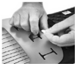
2. Place standard rivet head in slot
